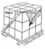
Diagram 2: Pull roll diagonally up to top of pallet.
