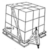
Diagram 3: Pull roll diagonally up to top of palles.
