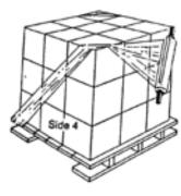
Diagram 4: Pull roll down and catch on pallet.
