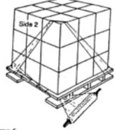
Diagram 6: Skip going up to top of pallet and go across bottom, catching on next corner.
